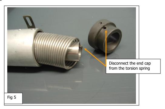
You should now be able to slide the roller tube off the assembly. When removing the roller tube, be sure to note how the canvas clamps are facing so you can reassemble the roller correctly later (the torsion springs only function correctly in one direction).
