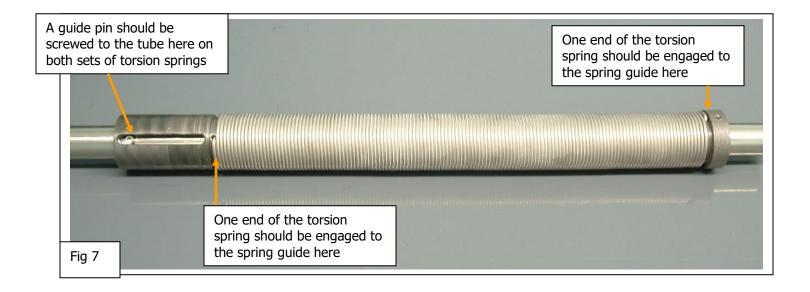
Reassemble the roller system and install back onto the actuators. Be sure that when you preload the roller that you only rotate the roller in the direction that the canvas comes off the roller.
