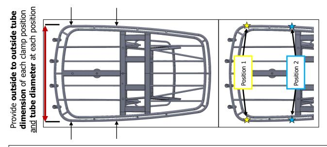
MTF shade width is specified by the **"outside to outside" tube dimension** – outside of PORT actuator to outside of STBD actuator. The maximum possible width for an MTF shade is 96" Once mounting area is determined for shade framework, measure and provide the OUTSIDE to OUTSIDE width dimension of both tubes the shade will be mounted to. Also measure and provide the diameter of both tubes.
