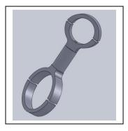
Spacers add extra length to the mounts to allow the shade to clear obstructions like rod holders and grab bars. SureShade can supply a spacer that extends the figure 8 clamp in  $\frac{1}{2}$ " (12.7 mm) increments up to 3" (76.2 mm). The shade framework is 4" (102 mm) tall. Measure the height of any obstruction in the path of the framework. Round the measurement up to the nearest  $\frac{1}{2}$ " (12.7 mm) to determine the height of the spacer required.
