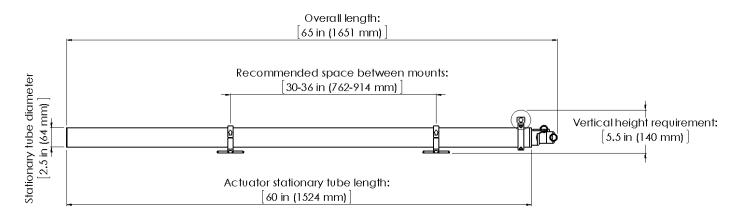
**STEP 2: DETERMINE SHADE WIDTH**. MTF framework (stationary actuator) and mounting clamps an **obstruction-free area** shown below.
