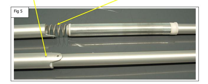
Finish reassembly by installing the components the same way you took the actuator apart to complete the updating of this actuator stage. **Be sure to use Loctite on screws when reinstalling.** Reattach crossbars and install the canvas to complete the Maintenance.
