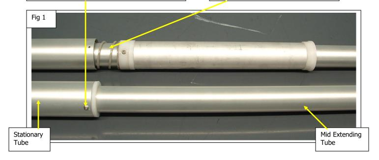
Reinstall the Mid Extending Tube into the stationary tube the same way you took the actuator apart to grease the springs in this actuator stage. **Be sure to use Loctite on screws when reinstalling.**
