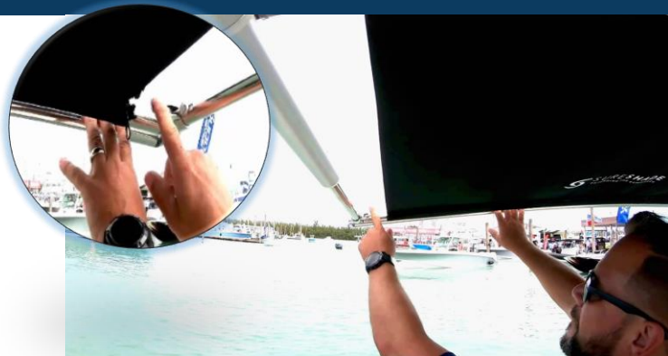
STEP 1 - Release levers on both sides of the shade; push shade out slightly as you push in lever
