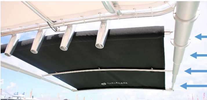
STEP 3 - Ensure 4 locking pins are locked in place on each side of shade
