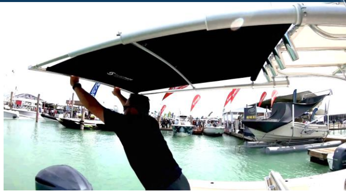
STEP 2 - Pull shade out evenly with constant momentum until shade is fully extended - RTX extends shade 4.5 feet
