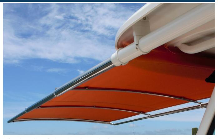
The SureShade® M3 automated mega shade system is an electric power-driven retractable shade featuring a self-supported stainless steel framework. The M3 features two crossbars enabling it to extend up to 10 feet.
